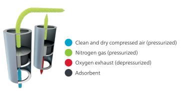
PSA technology isolates nitrogen molecules from other molecules in compressed air. Oxygen, CO<sub>2</sub>, water vapor and other gases are adsorbed. The result is virtually pure nitrogen at the outlet of the generator.
